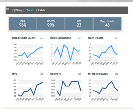
QDXray Quality assurance engine uses telemetry data from active network components to tag passive elements and infrastructure with KPI's.
